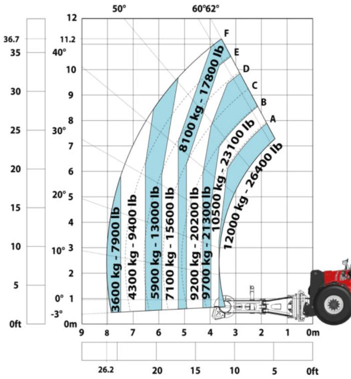
Machine on tyres with cylinder handler CH 10 (Metric)
