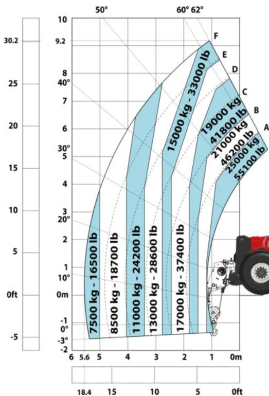
Machine on tyres with 3-hook jib 25000 kg (Metric)
