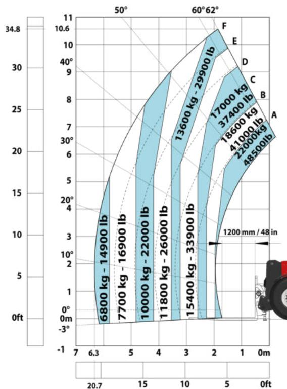
Machine on tyres with winch 25000 kg (Metric)
