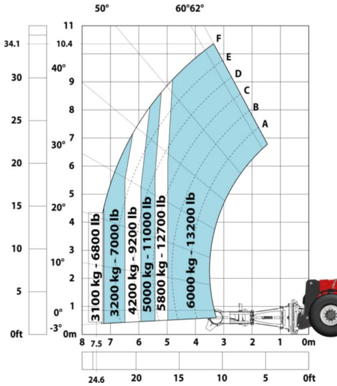
Machine on tyres with cylinder handler CH 10 (Metric)
